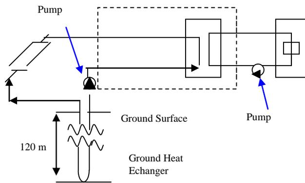
**Fig. 6:** Schematic of GSHP system coupled with solar collectors (summer cycle)
