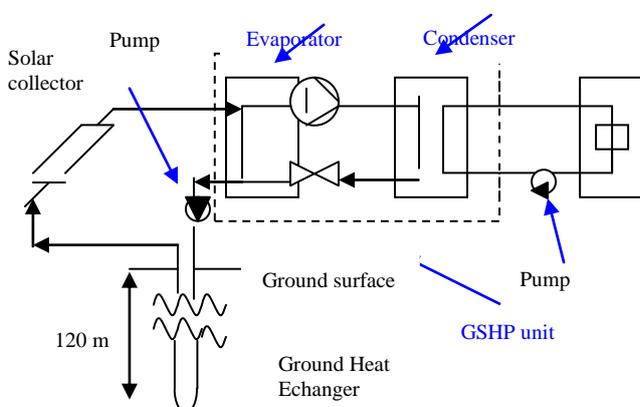
**Fig. 5:** Schematic of GSHP system coupled with solar collectors (winter cycle)
