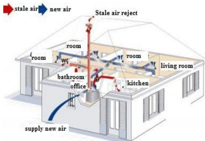
**Fig. 7:** VMC Double Flux Heat Recovery [7]
